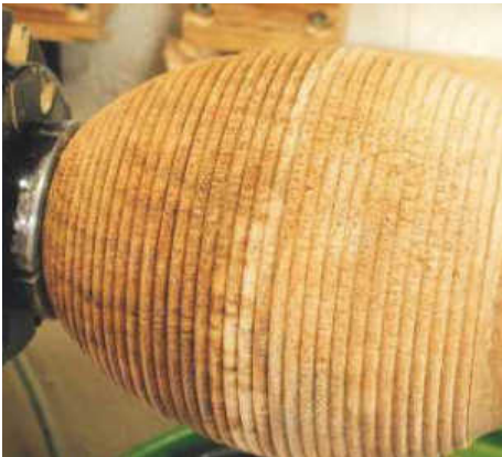
STEP 11. The problem with a bead scraper is that if the timber is a bit 'carroty', then they can break out, as they've done here. If you experience this, work on it later; see it as a texture rather than a problem
